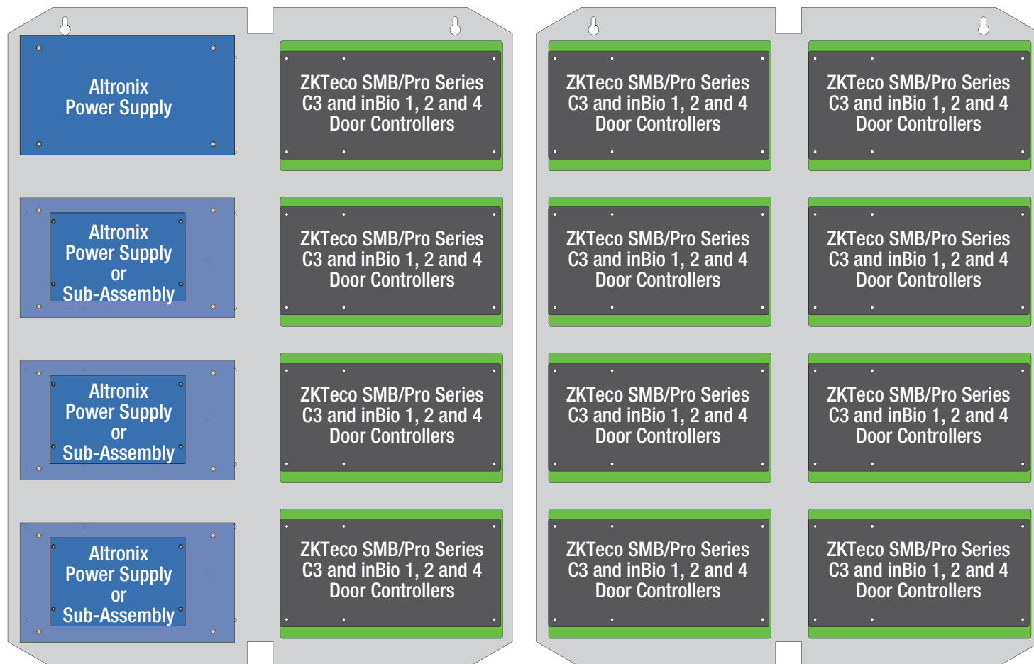
Trove2Z2 Interior Backplane - Optional Mounting Configurations
